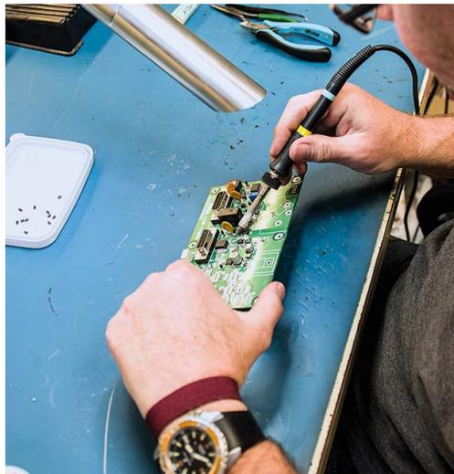
For small quantities, we are able to offer hand placement and soldering of Printed Circuit Boards, including Surface Mount components.
